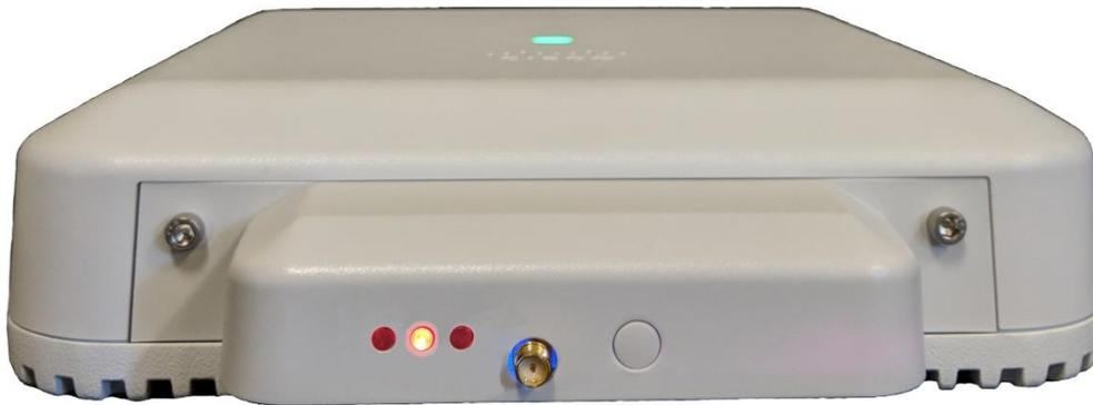
A solid blue light indicates the module is receiving power and is fully booted. This typically indicates normal operation.
