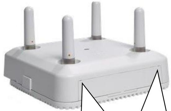
Using a small flathead screwdriver, release the snaps at both locations to remove the cover.
